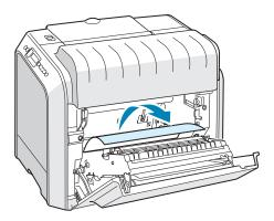
If there is any resistance, and the paper does not move immediately when you pull, stop pulling and go to step 3.
